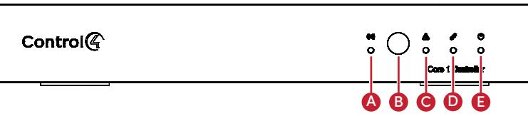
**A** Activity LED—The Activity LED shows when the controller is streaming audio.
