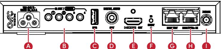
**A** Power port—AC power connector for an IEC 60320-C5 power cord.
