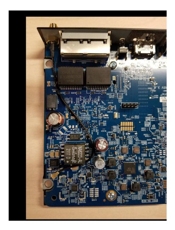
View of the 802.15.4 Transciever Circutry with RF Shield Removed
