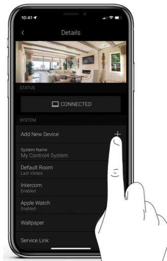
Scan the QR code in the Control4 mobile app by tapping the Control4 menu icon, going to Settings, selecting your system, then tapping **Add New Device**.
