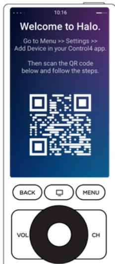
Press and hold the power button to turn the remote on. A QR code appears on the screen.
