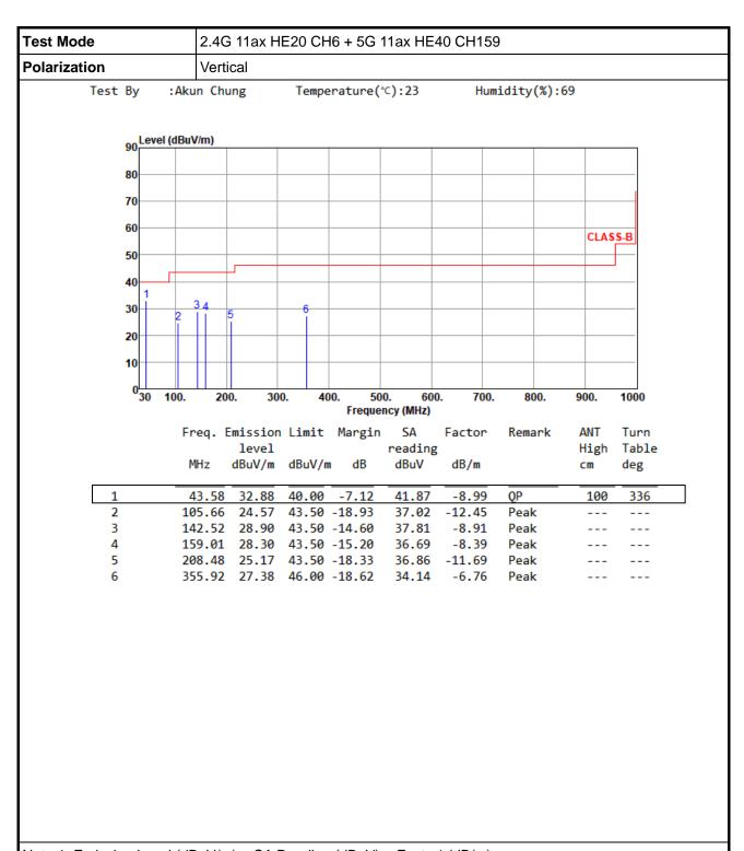
Note 1: Emission Level (dBuV/m) = SA Reading (dBuV) + Factor\* (dB/m)
