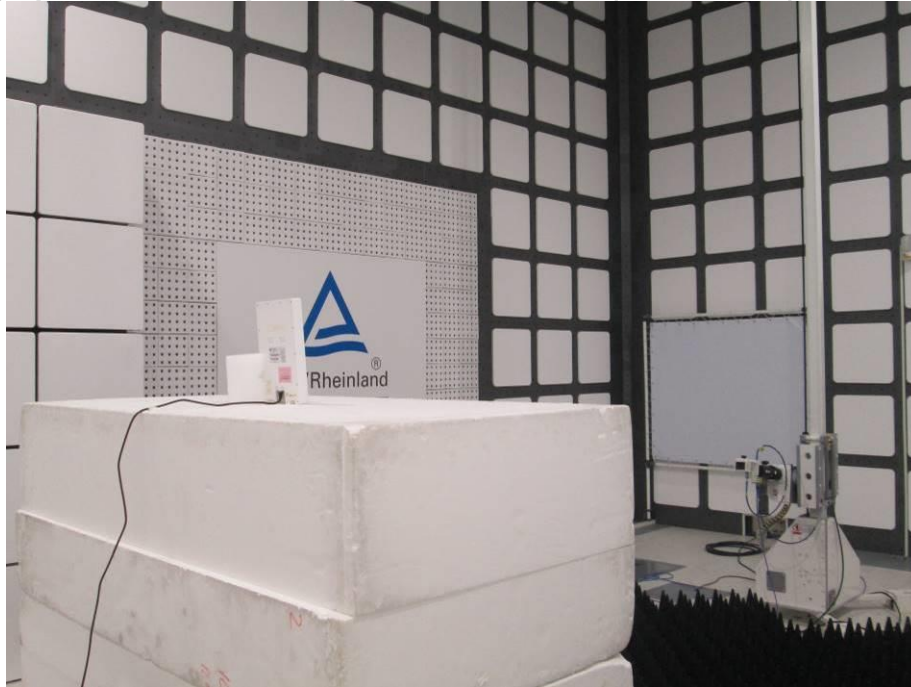
Photograph 6: Test Setup for Spurious Emissions (Back View 4)
