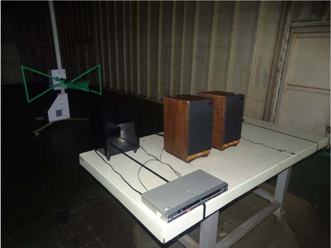
Front View of Radiated Test
