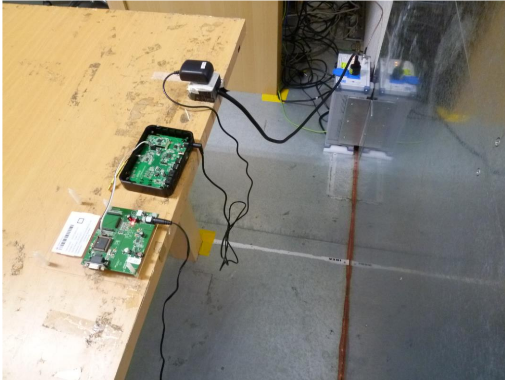
Photograph 7: Set-up for for Mains Conducted testing Front
