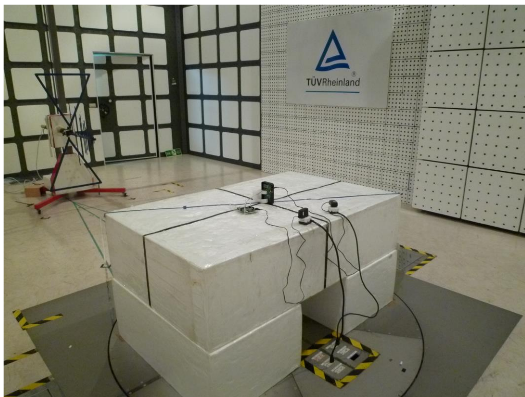
Photograph 3: Set-up for Spurious Emissions (Back View 2)
