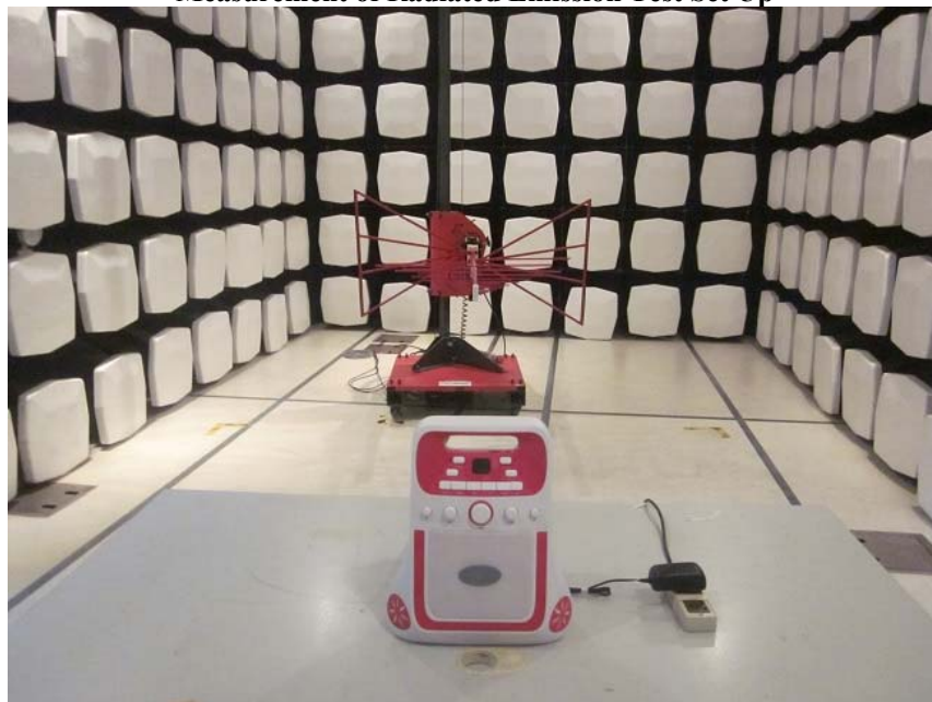
Measurement of Radiated Emission Test Set Up
