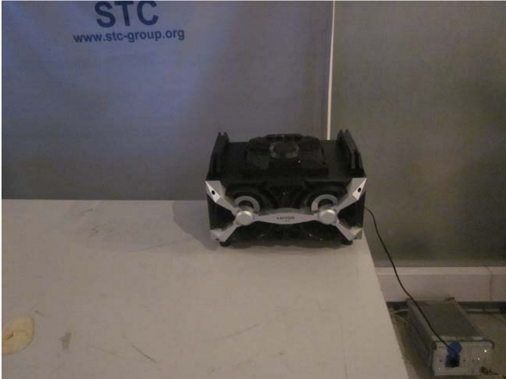
Measurement of Conducted Emission Test Set Up
