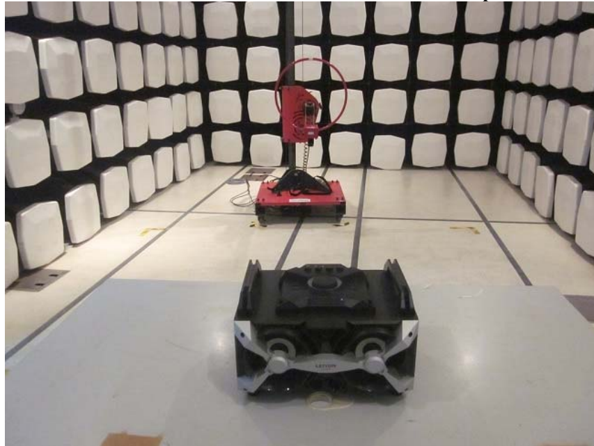
Measurement of Radiated Emission Test Set Up
