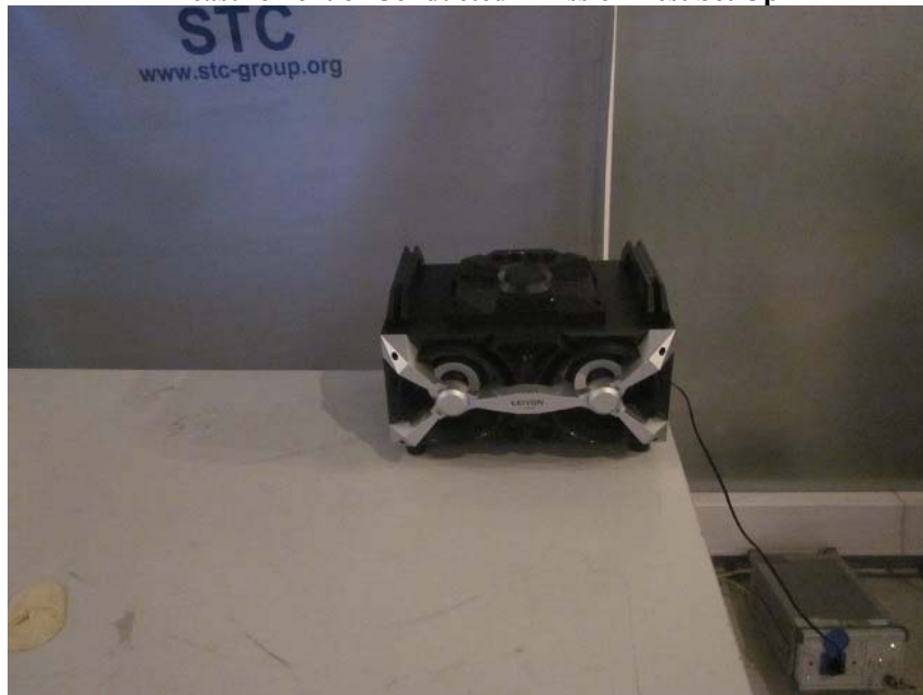
Measurement of Conducted Emission Test Set Up
