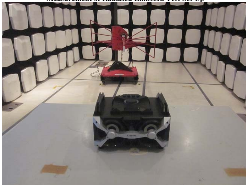
Measurement of Radiated Emission Test Set Up
