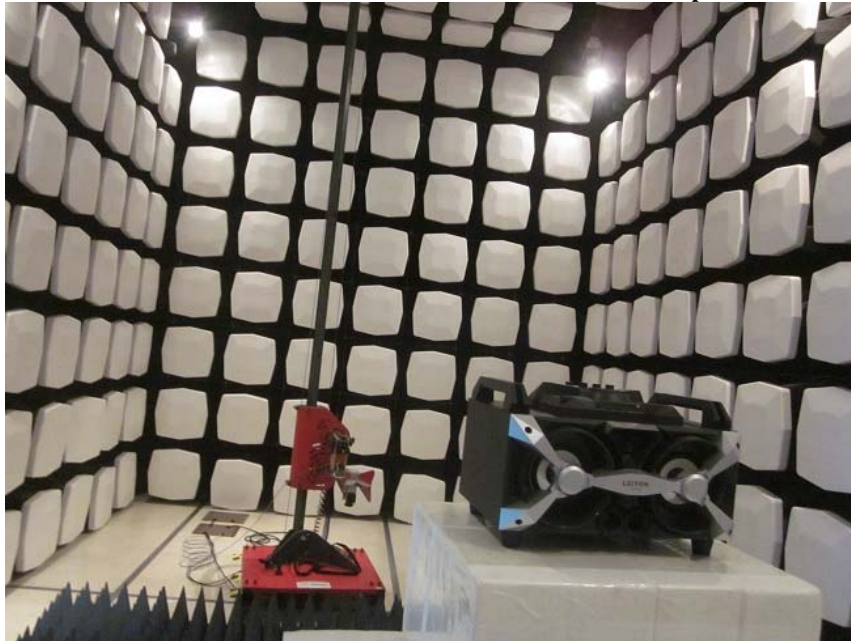
Measurement of Radiated Emission Test Set Up
