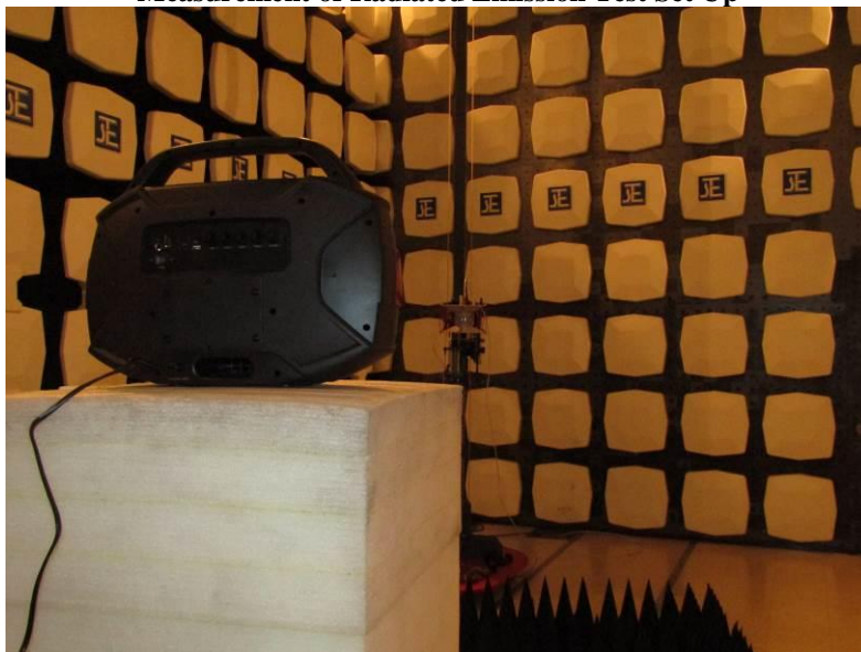
Measurement of Radiated Emission Test Set Up
