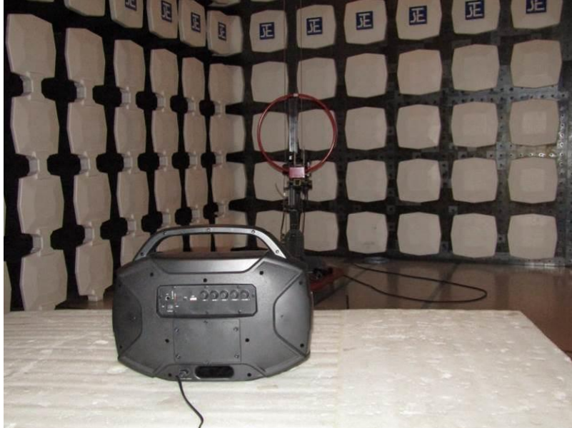
Measurement of Radiated Emission Test Set Up
