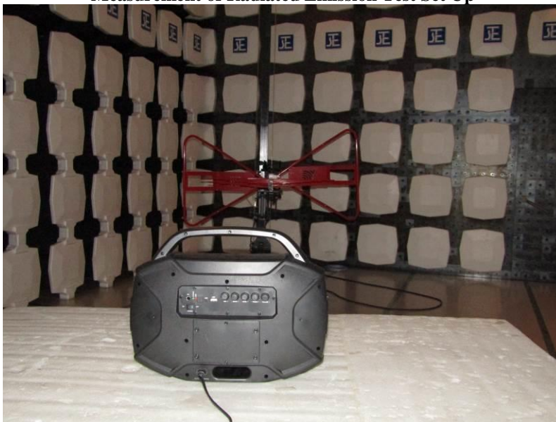
Measurement of Radiated Emission Test Set Up
