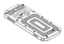
Note: When inserting the SIM card, ensure that the golden contacts faces right position.
