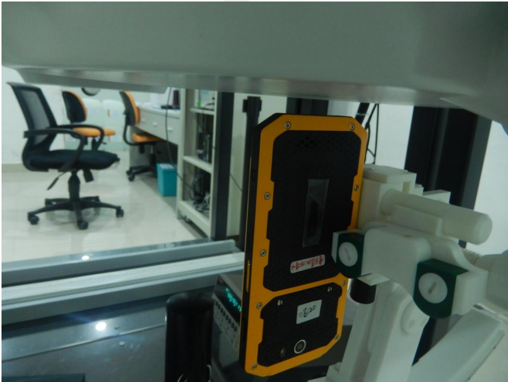
Body Bottom side(separation distance is 10mm)
