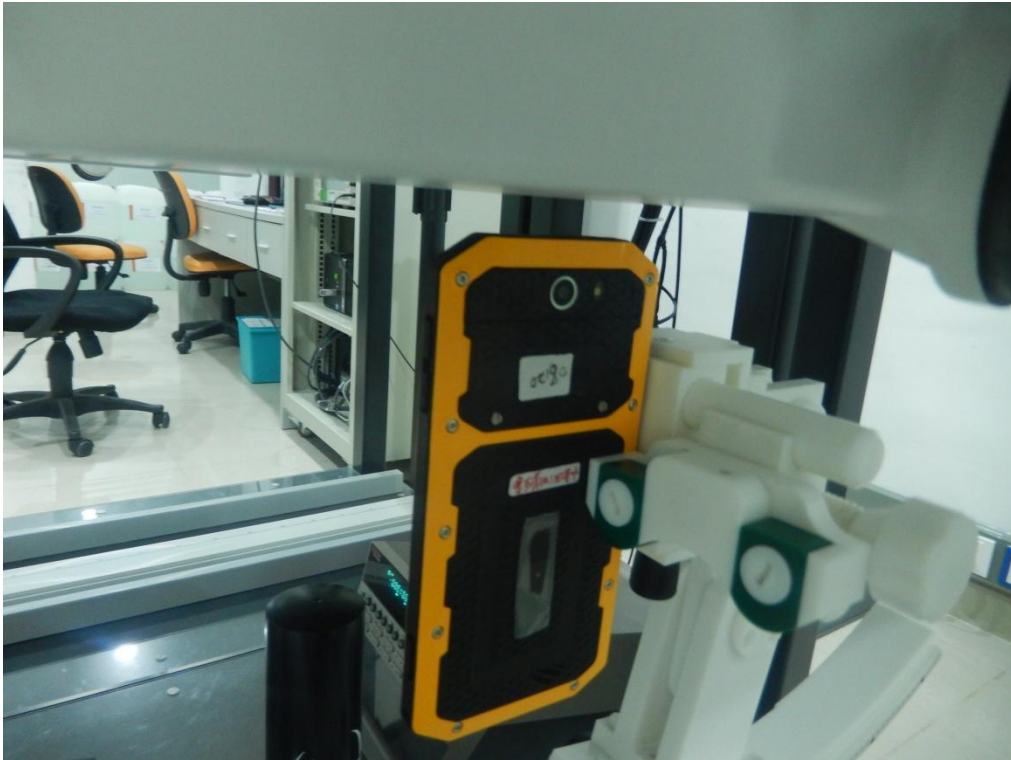
Body top side(separation distance is 10mm)
