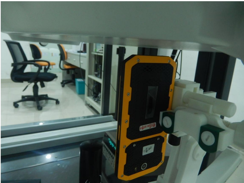
Body Bottom side(separation distance is 10mm)
