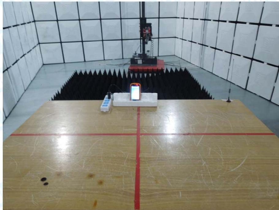
**Photo of Setup for Radiated Emission (Below 1 GHz)**
