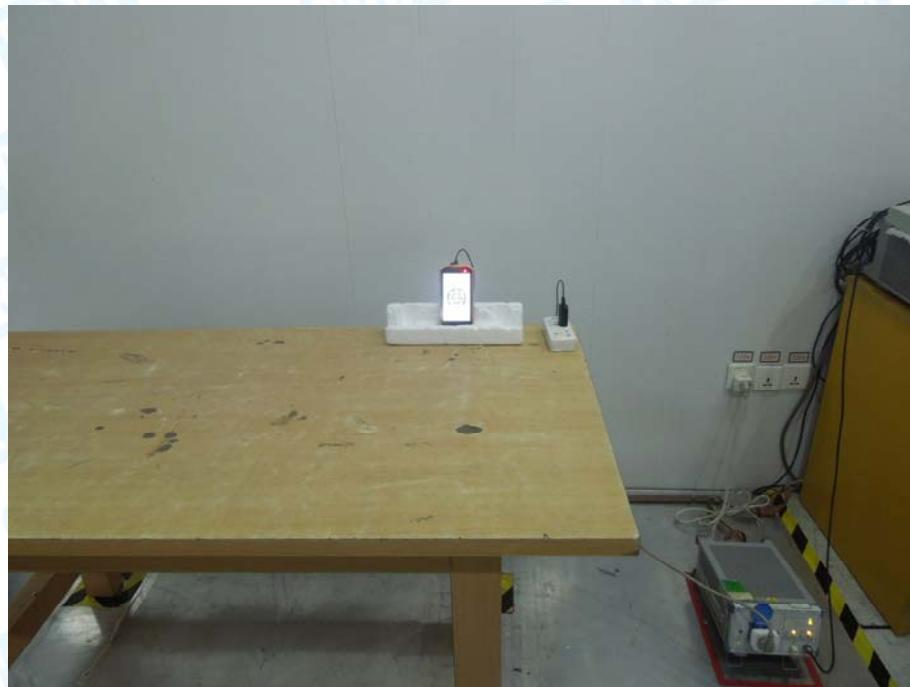
**FCC Part 22H&24E Test Setup****Photo of Setup for Radiated Emission (Above 1 GHz)**
