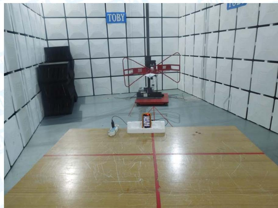
**Photo of Setup for Conducted Emission**
