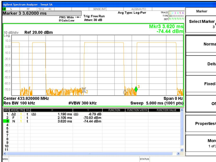
A manually operated transmitter shall employ a switch that will automatically deactivate the transmitter within not more than 5 seconds of being released.
