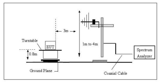
(C) Radiated Emission Test-Up Frequency Above 1GHz
