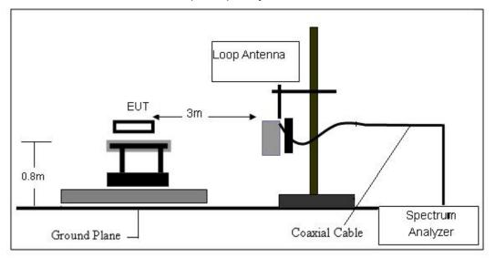
(B) Radiated Emission Test-Up Frequency 30MHz~1GHz
