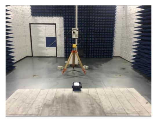
RADIATED EMISSION TEST SETUP BELOW 1GHz
