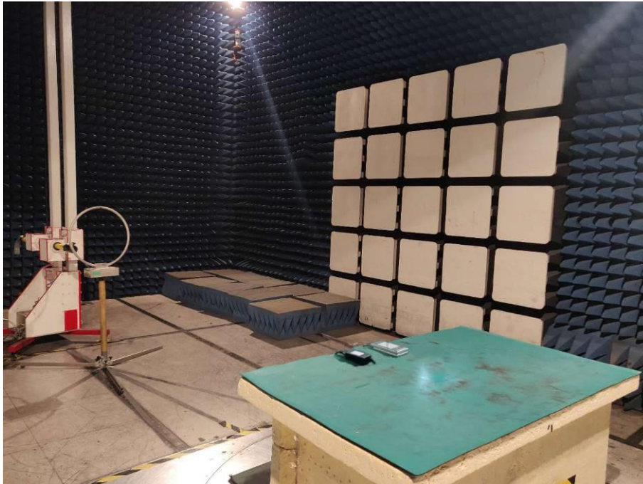
Spurious Emission Test Setup (Below 30MHz)
