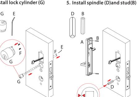
Note: Ensure the two triangles are in horizontal alignment.
