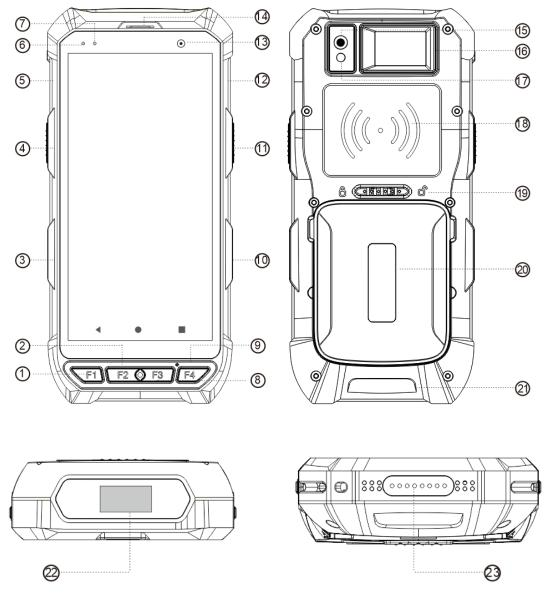
①F1 ②F2 ③Volume ④Reserved Button ⑤USB port ⑥Blue Led Indicator ⑦Red LED indicator ⑧F3 ⑨F4 ⑩Power Button ①Reserved Button ②Reserved Pogo Pin ③Front Camera ④Receiver ⑤Rear Camera ⑥Label ⑦Flashlight ⑱RFID Reading Area ⑨Battery Cover Locker ②Battery Cover ②Wrist Strap Locker ②Barcode Scan Window ③Cradle Pogo Pin Connector
