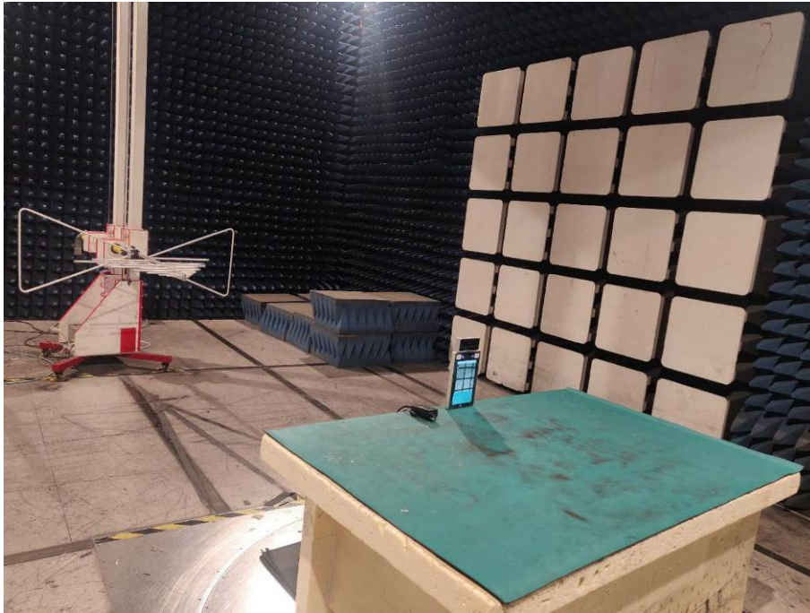
Spurious Emission Test Setup (30MHz-1GHz)
