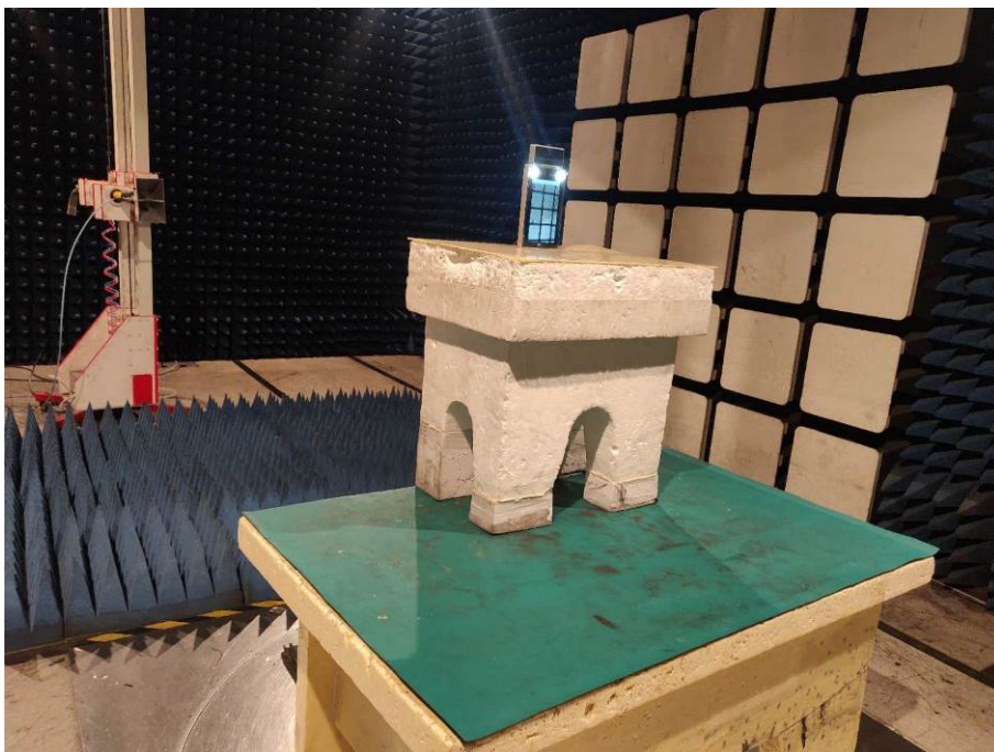
Spurious Emission Test Setup (Above 1GHz)
