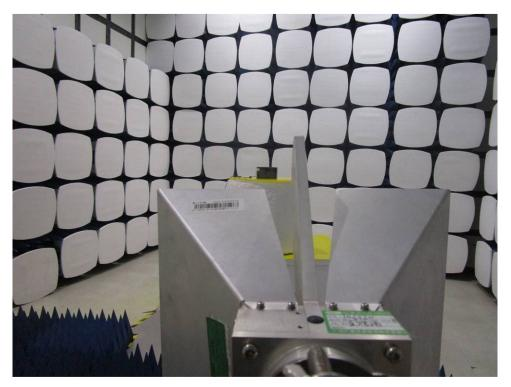
Radiated Emissions which fall in the restricted bands Test Setup
