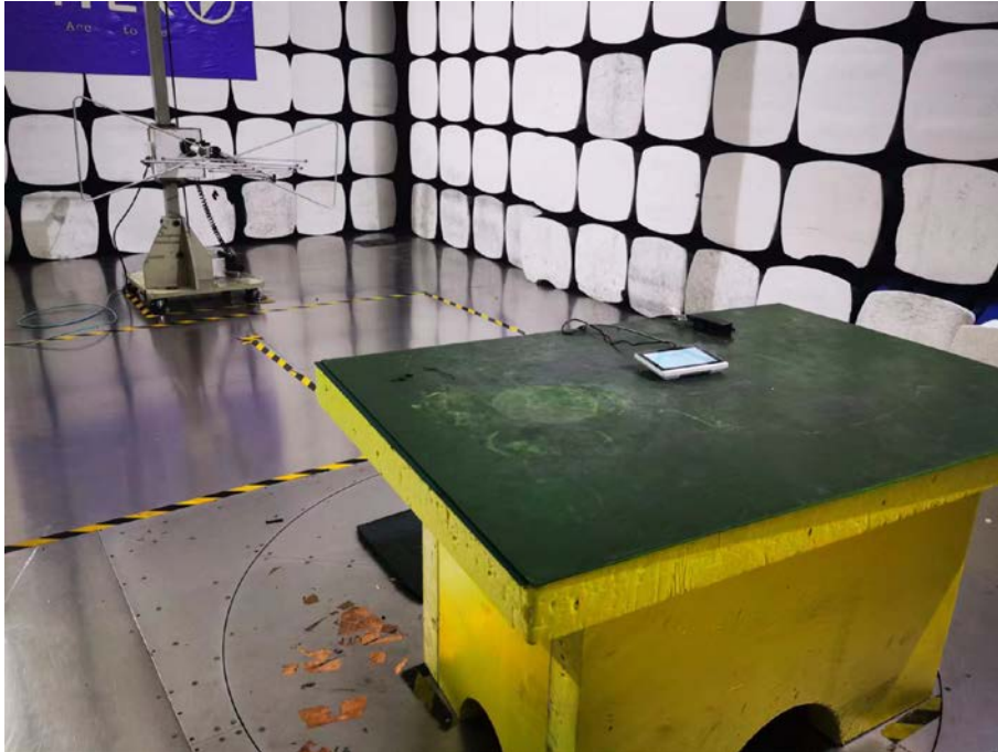
Spurious Emission Test Setup (Above 1GHz)
