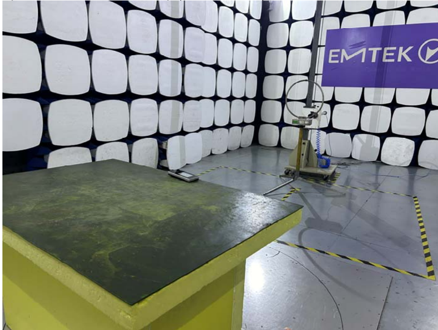
Spurious Emission Test Setup (Below 30MHz)
