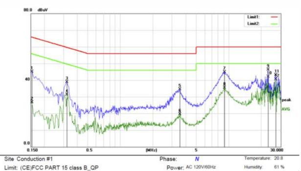
Limit: (CE)FCC PART 15 class B\_QP Mode: RFID (13.56M+125K) MODE
