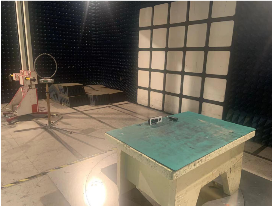
Spurious Emission Test Setup (Below 30MHz)
