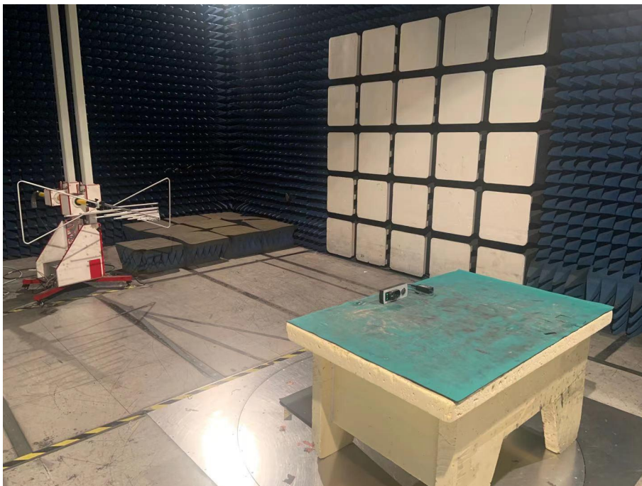
Spurious Emission Test Setup (30MHz-1GHz)
