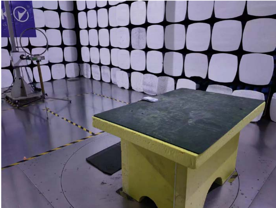
Spurious Emission Test Setup (Below 30Mhz)
