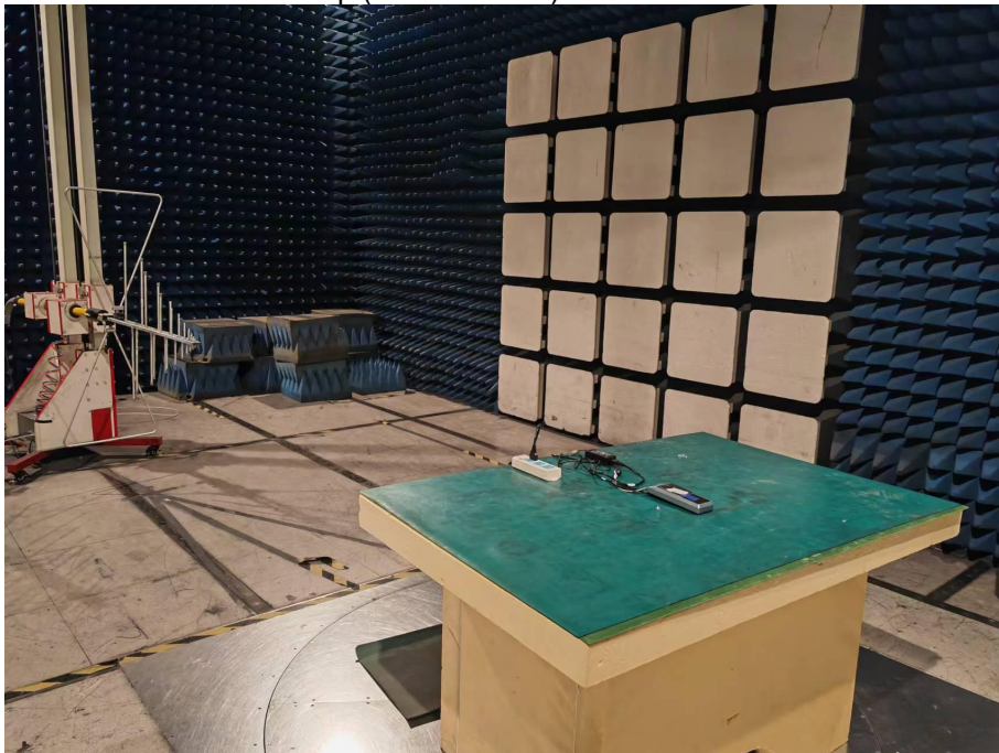
Spurious Emission Test Setup (30MHz-1GHz)
