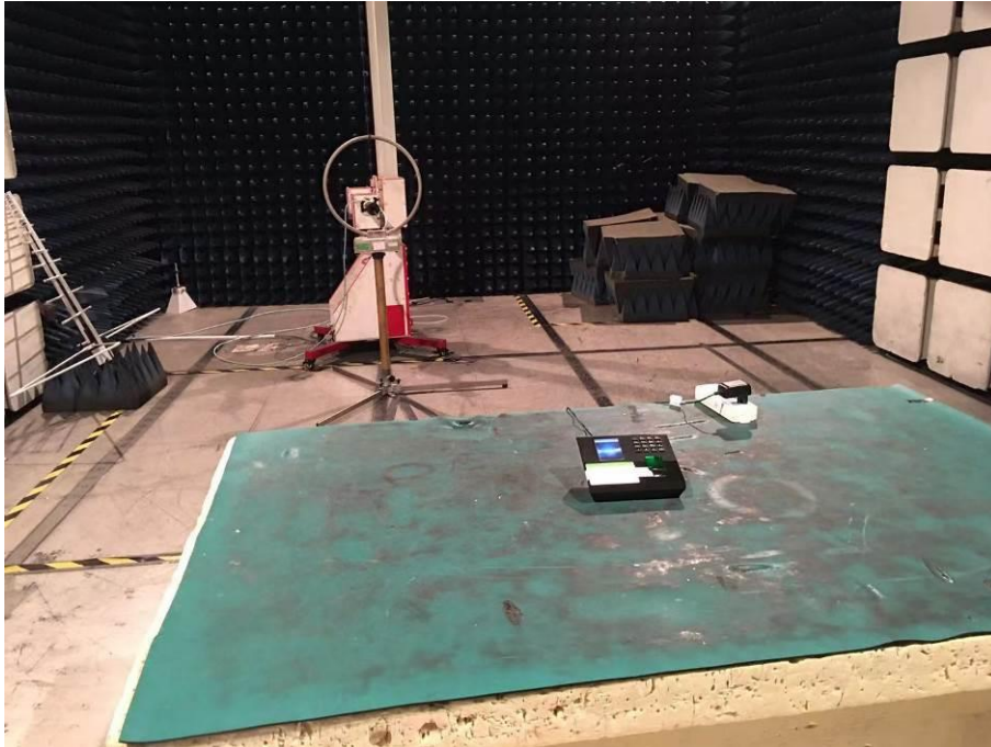
Spurious Emission Test Setup (Below 30MHz)
