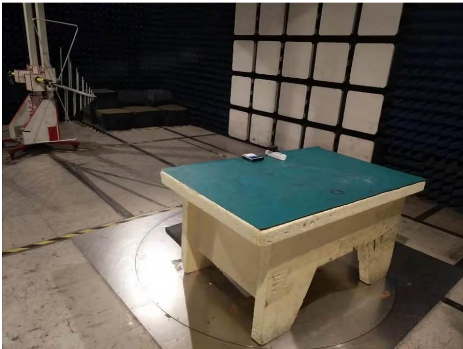
Spurious Emission Test Setup (30MHz-1GHz)
