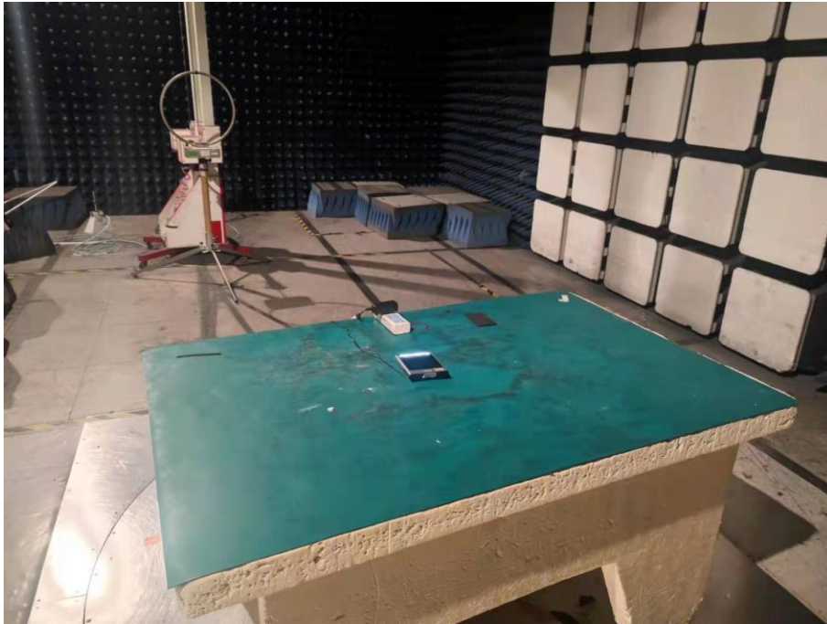
Spurious Emission Test Setup (Below 30MHz)
