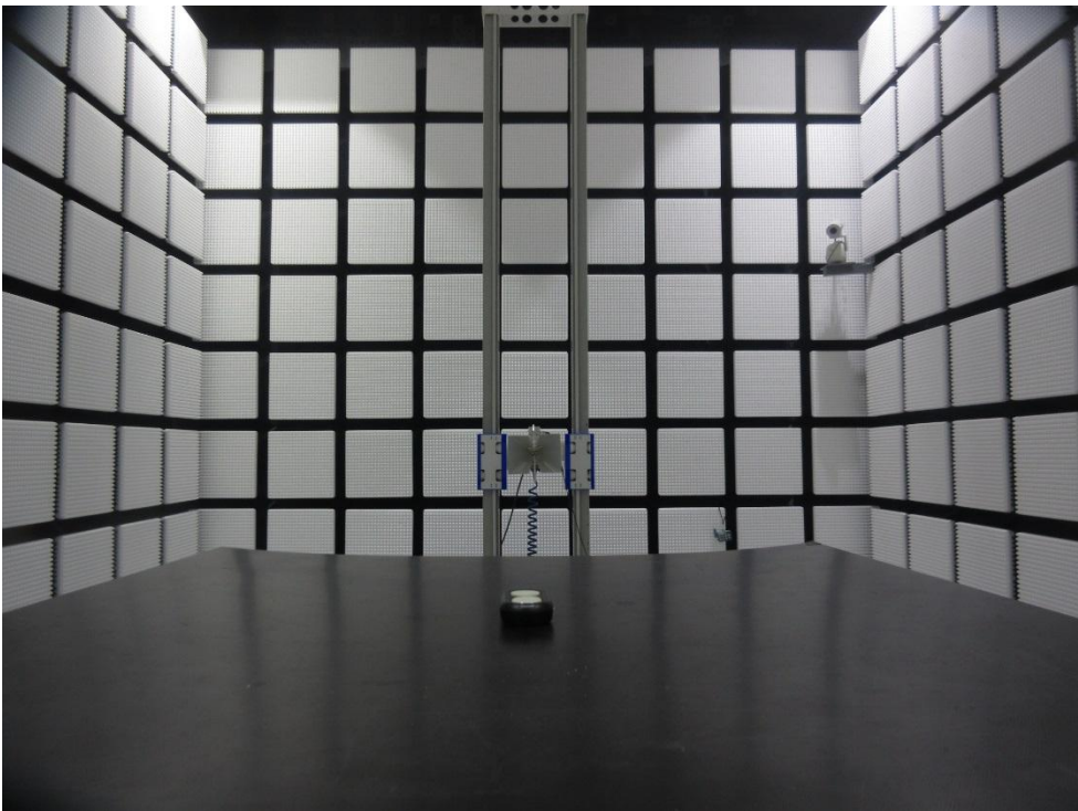
Radiated Emission Test Above 1GHz
