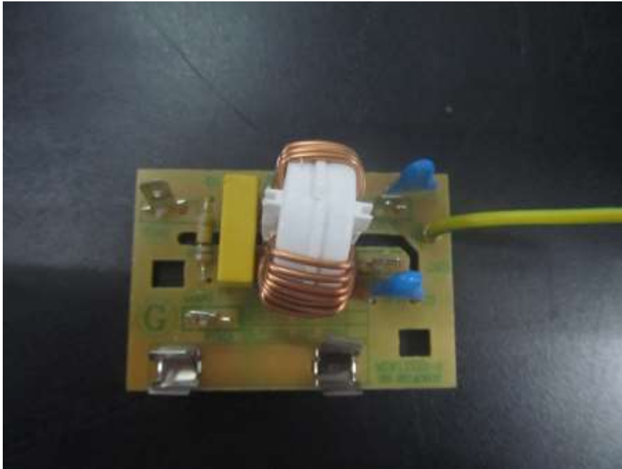
Power Filter Board Top View
