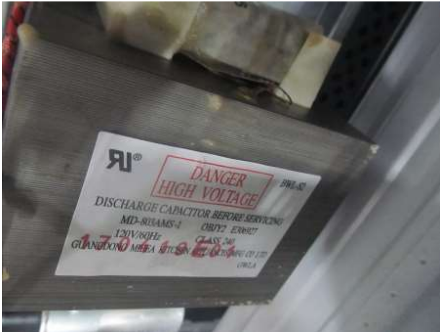
High-voltage Transformer view
