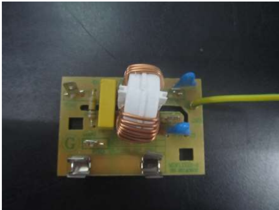
Power Filter Board Top View
