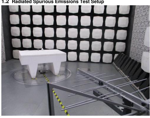
1.2 Radiated Spurious Emissions Test Setup
