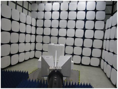
1.3 Radiated Spurious Emissions Test Setup
