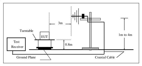
(c) For radiated emissions above 1000MHz
