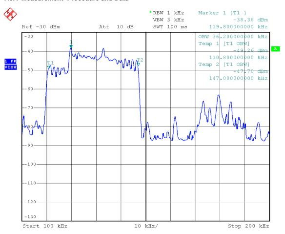
According the test data above, the fundamental wave is not fall in the restricted band 90kHz-110kHz, the field strength also meet the 15.209 requirement, please refer to section 7.3.
