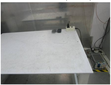
Radiated Emissions (9kHz-30MHz) Test Setup
