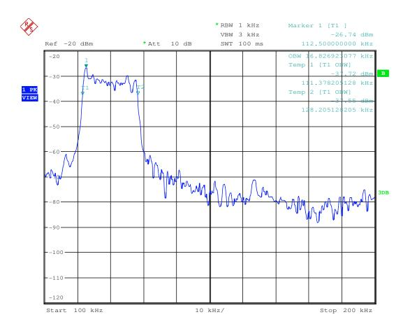
According the test data above, the fundamental wave is not fall in the restricted band 90KHz-150KHz, the field strength also meet the 15.209 requirement, please refer to clause 7.4.
