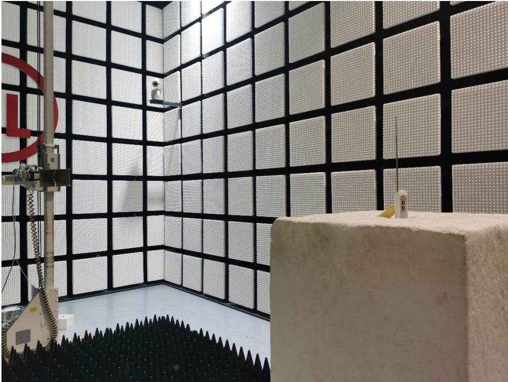
Radiated Disturbance Setup (Above 1 GHz – Z axis)
