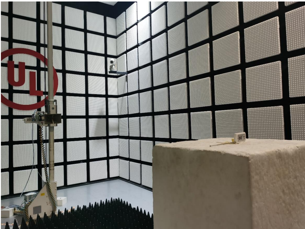
Radiated Disturbance Setup (Above 1 GHz – Y axis)
