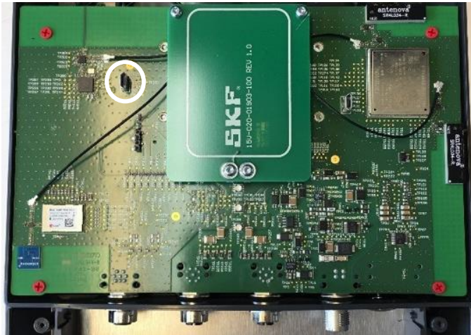
Figure 38 Location of USB service interface connector
