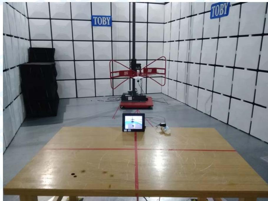
**Photo of Setup for Conducted Emission**
