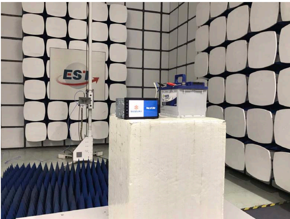
Radiated test: Above 1GHz
