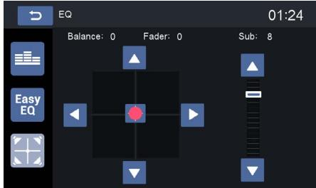
▶ Adjust fader and balance with [▼] / [▲] or [◀]/[▶].
