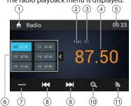
The radio display features the following functions and displays:
