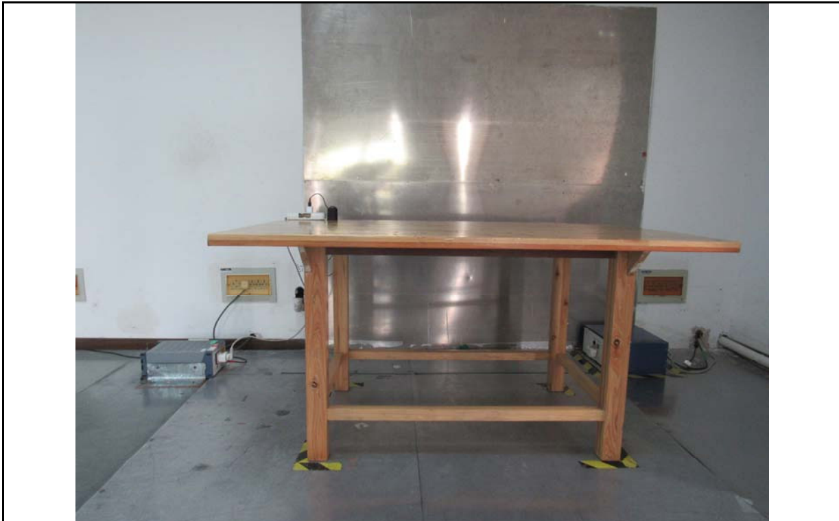
Conducted Emissions Test Setup Front View
