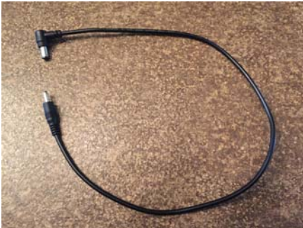
5. 90 Degree Cable Connector. Battery to PCB
