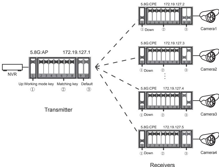
NOTE: For the point-to-point case, either of the four camera options above is available. Make sure the working mode key and matching Key are set right.
