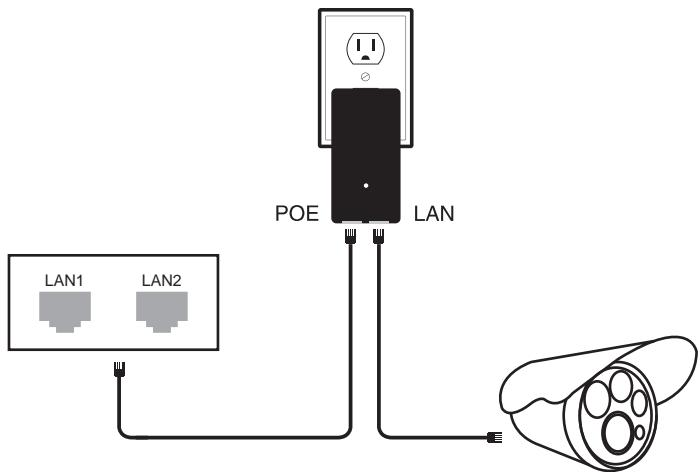
The bottom of the adapter has two RJ45 connections. One marked POE and one marked LAN.
