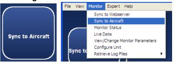
The Sync to Aircraft function is used to download log files from the monitor to the pc and to upload configuration files from the pc to the monitor
