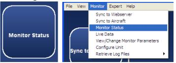
This function provides an overview of the status of the monitor and the status is updated continuously as long as the function is selected.
